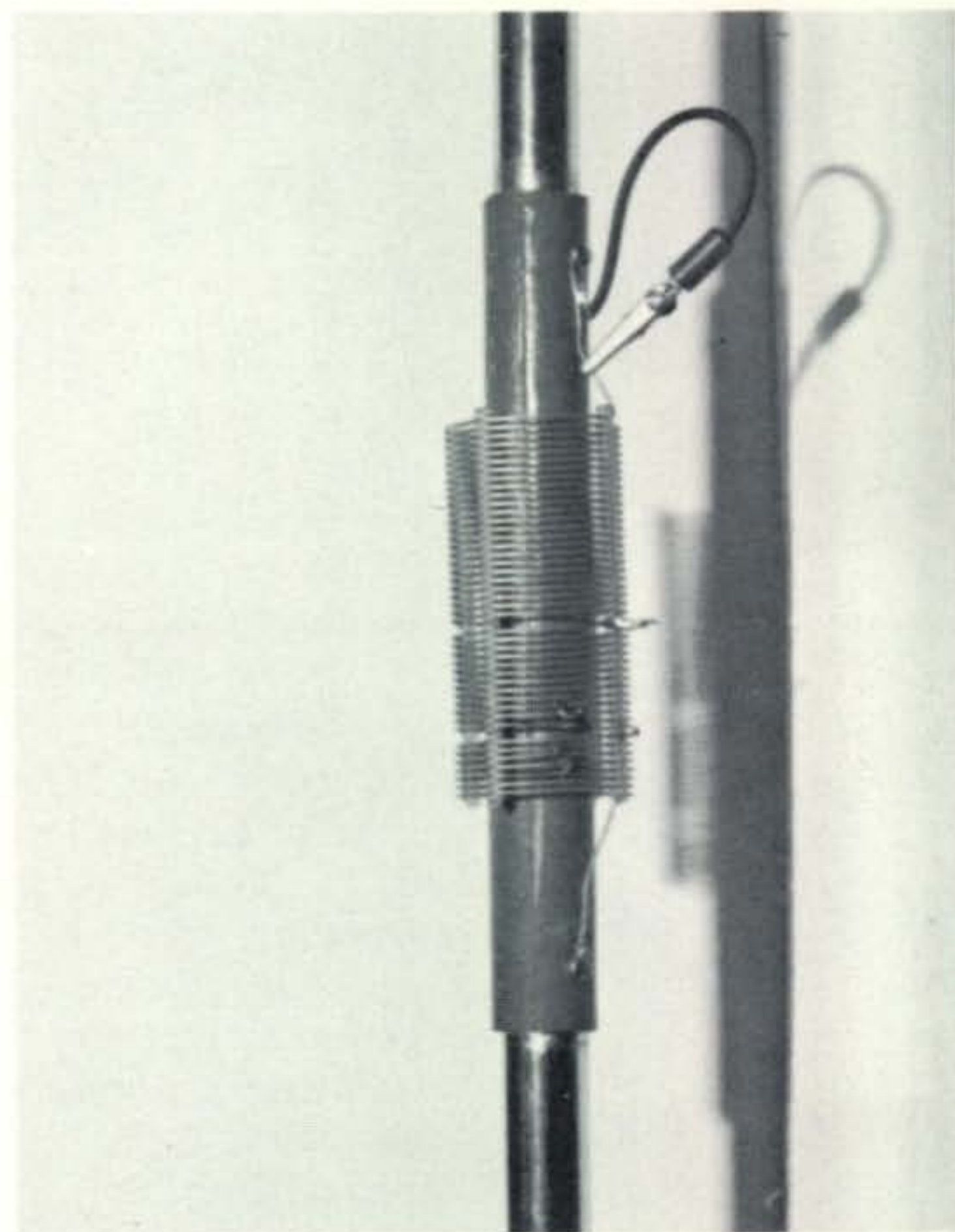
View of the center of the antenna shows the loading coil and the shorting clip. The antenna is usually turned to the wall so that the clip doesn't show.
