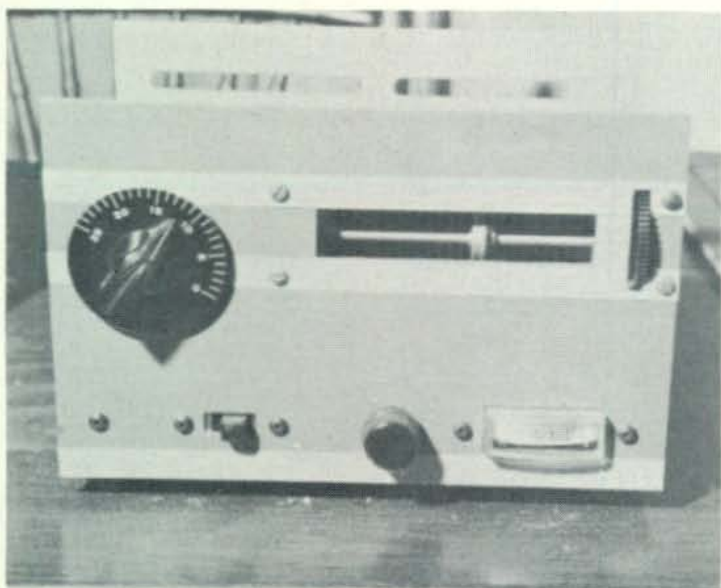
Front view of the L-net using the ARC-5 coil and a 250 mmf tuning capacitor. The s.w.r. bridge is built into the lower section of the L-net chassis.
